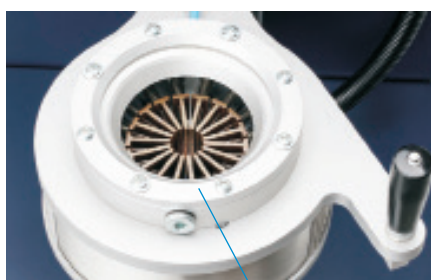
Circular nozzles for air cooling
